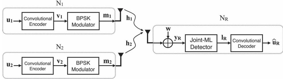
Fig. 1. Transmission/reception procedure of multiple access phase in PNC with CCs.
